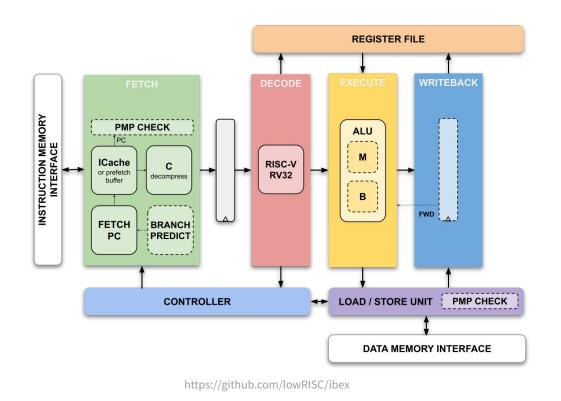
Highly configurable **open source** RV32IMCB core with security features that include:
